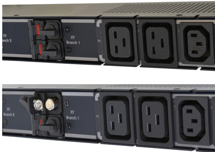
Figure 15. Partial views of fused rack PDU utilizing CCPLP with SC fuses. This rack PDU uses SC fuses to protect the receptacles and circuit to the power supplies. Courtesy of Server Technology, Inc.
