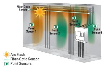
Scenario with point sensor placement on the wall of each compartment. Arc detection area for each sensor is shown in green shade. In this case, both Point Sensor 1 and the Fiber-Optic Sensor detected the flash as it was within their viewing area (shown in orange).
