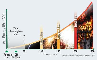
The Littelfuse Arc-Flash Relays use a 125-µs light-sampling scheme in combination with an ultra-fast IGBT output to be able to detect a developing arc flash and send a trip signal to a circuit breaker in less than 1 ms.
