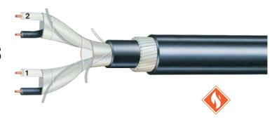
**Construction** Plain annealed copper conductor, V-90RP PVC insulated, twisted pairs individually & overall screened with aluminium polyester tape plus tinned copper drain wire, rip cord, PVC bedding, steel wire armour, V-90RP PVC sheathed.
