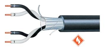
**Construction** Plain annealed copper conductor, V-90RP PVC insulated, twisted pairs, unscreened or overall screened with aluminium polyester tape plus tinned copper drain wire, rip cord, V-90RP PVC sheathed.
