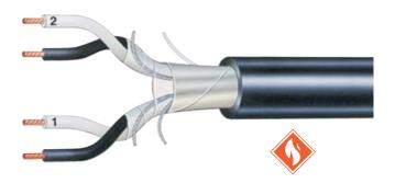
**Construction** Plain annealed copper conductor, V-90RP PVC insulated, twisted pairs, individually and overall screened with aluminium polyester tape plus tinned copper drain wire, rip cord, V-90RP PVC sheathed.
