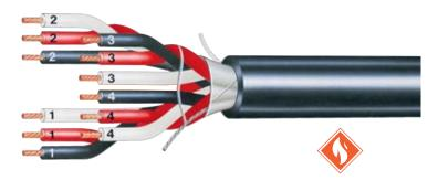
**Construction** Plain annealed copper conductor, V-90RP PVC insulated, twisted triples, unscreened or overall screened with aluminium polyester tape plus tinned copper drain wire, rip cord, V-90RP PVC sheathed.
