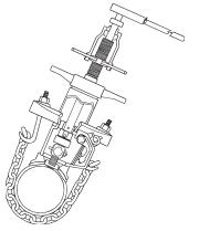
The drilling and tapping tool is extracted and a corporation stop is attached to the boring bar for insertion into the main.
