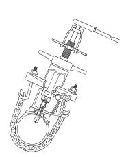
MUELLER drilling and tapping machine drills and taps a hole in a pressurized main without allowing water to escape.
